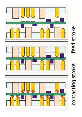
The **2-stroke adapter** offers the great advantage that, with the feed stroke, the substrate is supported by the push rods in a stable manner and no force is exerted on the substrate.
