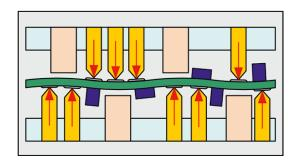
In the case of the **1-stroke adapter**, the spring probes already exert their contacting force before the push rods can support the substrate. In this state, this leads to a deformation and thus to a greater load on the substrate.
